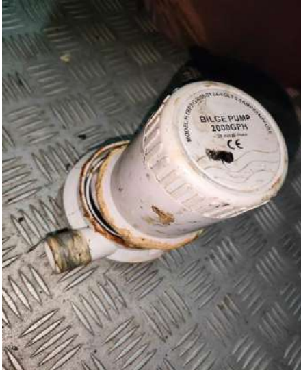
Bilge Submersible Pump, 24Volts
